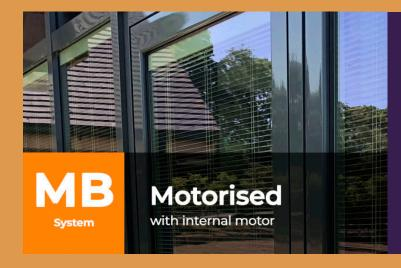
The MB system is a 24 volt hard wired system. The system is operated via a remote control, push button or our app. Leaving nothing on the outside of the glass, this system gives the ultimate finish. The most common application for the MB system is high end residential projects and the system is ideal for bi folding or sliding doors
