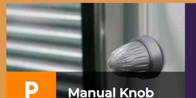
The P System is a manual operated system for venetian blinds incorporated within a 20 or 22-mm cavity. It is designed to perform a tilt-only function of the blinds by means of an external knob that is secured to the window frame: the glass appears completely clear, easy to be clean and free from external devices.
