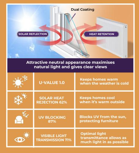
\*Based on a unit construction of 4mm custom ambient toughened / 16mm argon filled cavity / 4mm clear toughened
